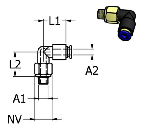
Ext. hose diameter A2 = 4 mm L1 = 14 L2 = 17.2 NV = 8 Thread A! = M3
